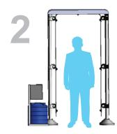
Sensors detect the presence of human and triggers the spraying mechanism for 10 seconds.
