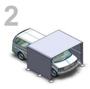
Sensors detect the presence of the vehicle and triggers the spraying
