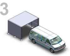
As the car has completely driven through the kiosk the spraying stops as the sensor does not detect the presence of the vehicle.
